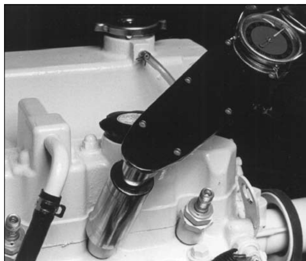
Figure 14: Reinstall injector. Torque to proper tightness.
